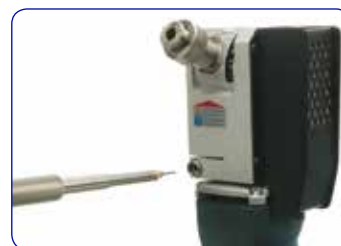
Precise adjustment of the stick-out
