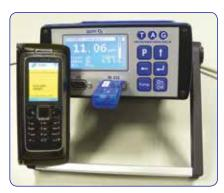
Connected via a Bluetooth Dongle with a range of up to 100m to a mobile phone. Via the phone all relevant data including rest oxygen level, sensor temperature will be displayed. Using simple commands the PRO PURGE 1 can be operated remotely
