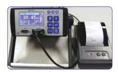
Connecting a printer via the RS232 interface. Capable of readout documentation (per second) that can be logged via a printer
