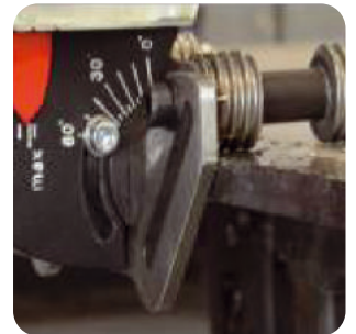
Continuous angle adjustment from 0 to 60 degrees.
