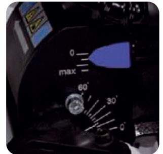
Continuous angle adjustment from 0 to 60 degrees.
