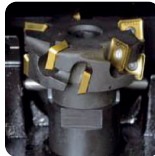
Mono block milling head, with 10 indexable inserts fixed with screws.
