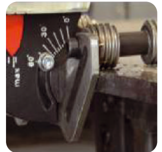
Continuous angle adjustment from 0 to 60 degrees.
