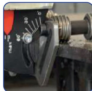
Continuous angle adjustment from 0 to 60 degrees.
