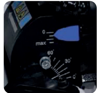
Continuous angle adjustment from 0 to 60 degrees.
