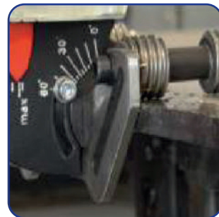
Continuous angle adjustment from 0 to 60 degrees.
