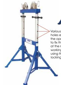
Various height holes enable the operator to fix the stand at the required working height using the safety locking pins
