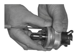
3. Tighten the two screws on the cover plate and check the adjustment either by measurement across the pins or by forming a trial outlet.
