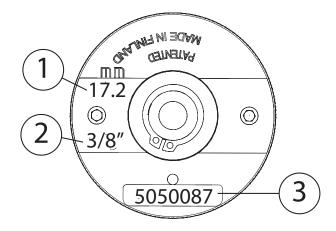
Identification: 1. Actual size in millimetres, 2. Nominal size in inches (NS), 3. The ordering and identification number of the T-DRILL head
