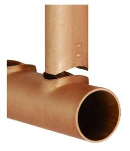
7. Align dimples with the run of the tube after insertion into the outlet. Braze the joint.
