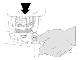
11. Start forming the outlet by pulling the trigger and continue until the T-DRILL head is completely out of the tube. During the forming of the tee, keep the tube support against the tube and push the tool toward the tube. This insures that you obtain a circular outlet.
