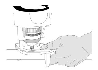
7. Pull the support legs out and place the tube support firmly onto the point where the tee is to be formed on the tube, as shown on the illustration. Press the tube support with the thumb against the tube and twist the machine counterclockwise at the handle of the tool. This centers the T-DRILL head onto the tube.
