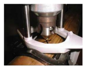
4. Retract forming pins on T-DRILL Head and attach T-DRILL T-65 to counterplate. Notches on tube support fit on tabs of counterplate.
