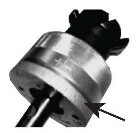
2. To enlarge the outlet rotate the conical cover with respect to the cover plate in plus (+) direction. Hold the cover plate stationary.
