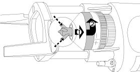
5. Retract forming pins. Press the conical cover towards the tool and rotate it clockwise to retract the forming pins.
