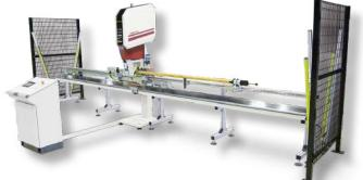
S-54 AFT S-54 collaring unit with Automatic Feed Table (AFT).
