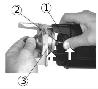
Chucking the T-DRILL head and removing it.
