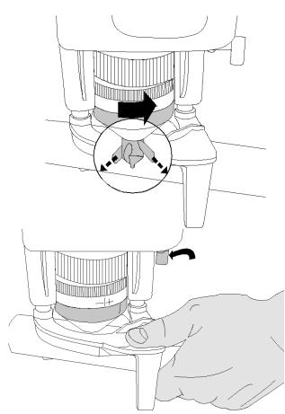
9. Extend the forming pins on the T-DRILL head by pressing the conical cover towards the tool and rotating it counterclockwise until the T-DRILL head locks into the tee forming position.
