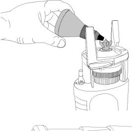
4. Lubricate the T-DRILL head before every tee forming operation! Extend the forming pins and lubricate them as well as the cutting edges of the T-DRILL head as illustrated. Always use T-DRILL lubricant.
