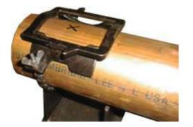
2. Attach counterplate to the tube where annealing has been done.
