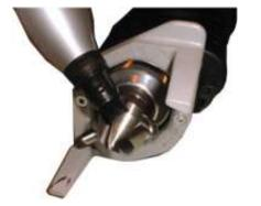
3. Lubricate forming pins and cutting edges on T-DRILL head.
