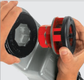
Easy insertion of the die heads
