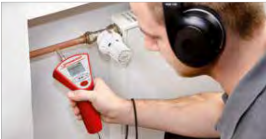
Acoustic leak detection of heating installations
