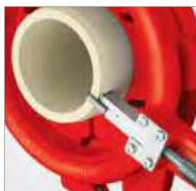
ROCUT 160 with cutter blade
