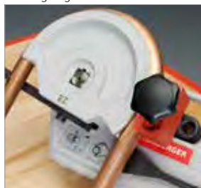
Forged aluminium segments with bending angle scale
