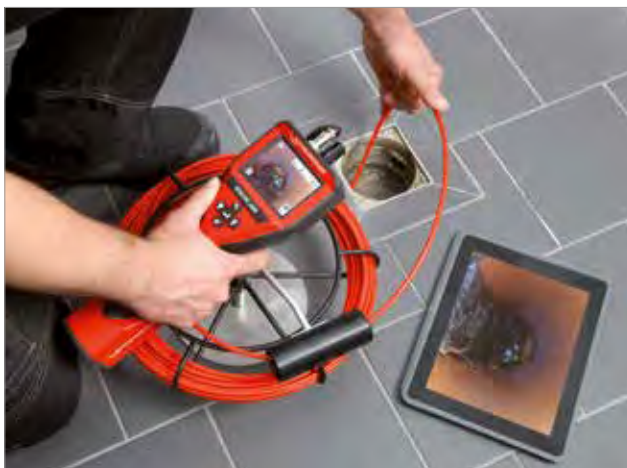
Inspection of basin drains
