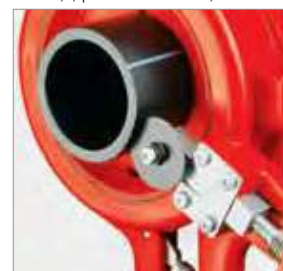
ROCUT 110 with cutter wheel (No. 54950) (special accessories)
