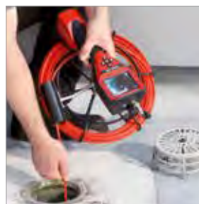
Inspection of rain downpipes
