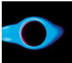
High flame temperature based on cyclone swirl
