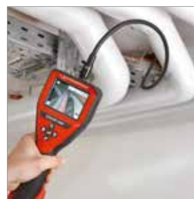
Inspection of hollow spaces
