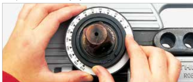
Pre-adjustment of the bending angle without tools
