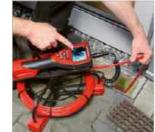
Inspection of rain drainpipes
