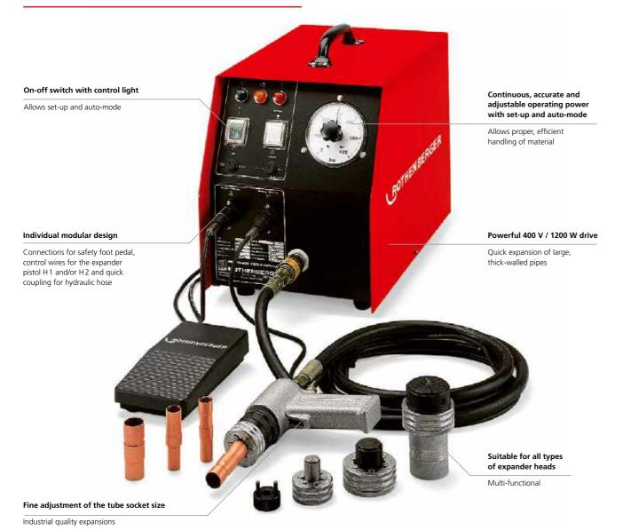
Set (No. 13100) includes: Electro-hydraulic expander system H 600 complete with hydraulic unit H 600 (No. 13002), expander pistol H1 (No. 12001), control cable, hydraulic hose 2.5 m with circuit points, adjusting tool, tool rack (No. 13023), safety foot pedal and hydraulic oil 1 l (No. 58185), without expander heads
