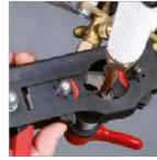
Automatic depth stop: perfect positioning of the pipe to the flare cone
