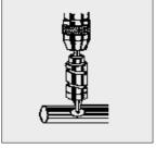
Insert extractor hook into the drilled hole and screw the bell
