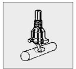
Using the ratchet, turn the extractor to the left, while paying attention that the V-block is seated securely
