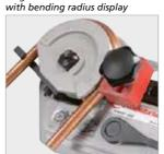
Pre-adjustment of the bending angle without tools
