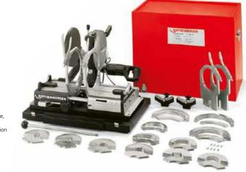
**Set (No. 55795) includes:** holder for heating plate, electronically adjustable heating plate, basic clamping set Ø 160 mm and 250 mm support fork inserts Ø 160 mm and 250 mm, reducer inserts and support fork inserts from Ø 40 - 140 mm and Ø 180 - 225 mm, installation tools, steel transport box 800 x 520 x 765 mm (LxWxH) and steel carrying case for reducer and support fork inserts
