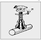
After extraction, set correct insertion depth (dependant on
