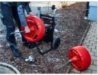
automatic spiral feed for removal of blockages in pipes from
