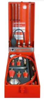
Testing scale up to 150 mbar on transparent extending tube element
