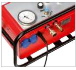
Electronic control for heating element can be placed flexibly using a magnet (P 355 B)
