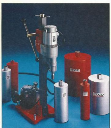
RIDGID Core Drills cut clean, round holes from 1/2" to 14" diameter in reinforced concrete, masonry and other hard materials; for installing pipe, electrical wires, vents and anchors for machines.
