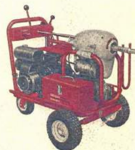
K-2000 Municipal Sewer Cleaner Recommended for clearing municipal sewer lines 6" to 10" diameter to 250' using sectional cable and through 24" mains to 500' using solid rods
