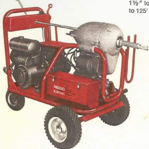
K-2000 Municipal Sewer Cleaner Recommended for clearing municipal sewer lines 6" to 10" diameter (to 250' using sectional cable) and through 24" mains (to 500' using solid rods)
