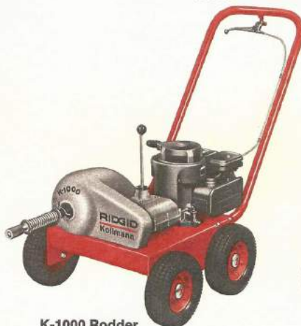
K-1000 Rodder Recommended for small municipalities, factory complexes, campuses, institutions, golf courses with lines through 24" diameter to 500'
