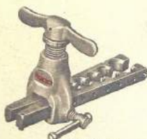
Flaring Tools Six models for 45° and 37° flares
