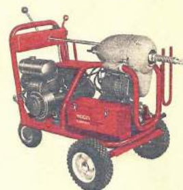
K-2000 Municipal Sewer Cleaner Recommended for clearing municipal sewer lines 8" to 16" diameter to 250' using sectional cable and through 24" mains to 500' using solid rods
