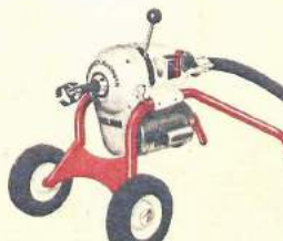
KM-1500 Drain Cleaner Recommended for clearing 1 1/2" to 8" diameter lines to 200'
