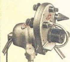
No. 124 Copper Cleaning Machine Cleans • Reams • Faces
