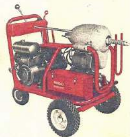
K-2000 Municipal Sewer Cleaner Recommended for clearing municipal sewer lines 8" to 12" diameter to 250' using sectional cable and through 24" mains to 500' using solid rods
