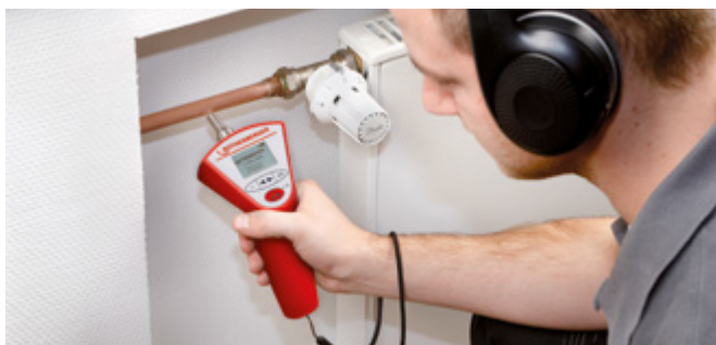
Acoustic leak detection of heating installations
