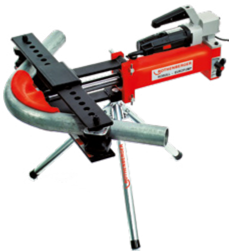
ROBULL type ME with foldable bending frame
