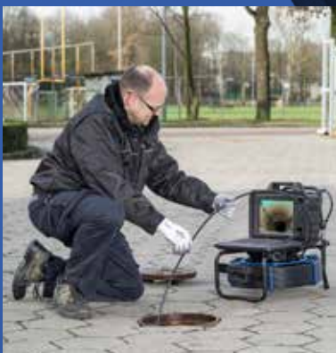
Rioned FlexCam with self-levelling camera head
