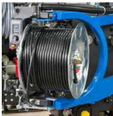
Pivoting and rotating hose reel
