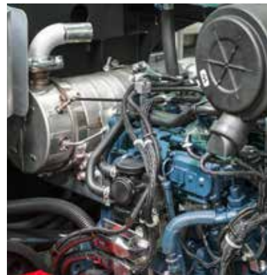
Tier 4/stage V ready engine with built-in diesel particle filter
