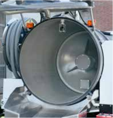
Movable partition for capacity increases
