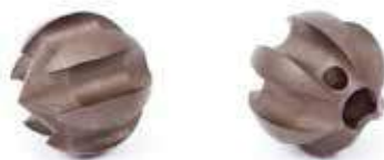
11 TULIP CUTTER The Tulip Cutter causes less damage, never gets stuck and removes debris more evenly, safely and cleanly than similar tools, such as a chain head. Ideal for removing hardened grease, lime and urine deposits and rust in pipes ranging from 50 to 125 mm.
