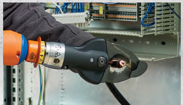
VDE-standard battery-powered hydraulic cutting tool ESM 50 IS
