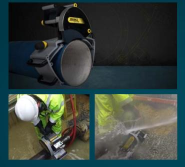
For greater cutting depth there is an option to purhcase 180 mm blades. Available models: **Diamond X 180** – cast iron, **Cermet 180** – stainless steel, carbon steel, **ALU 180** – plastics and aluminium.
