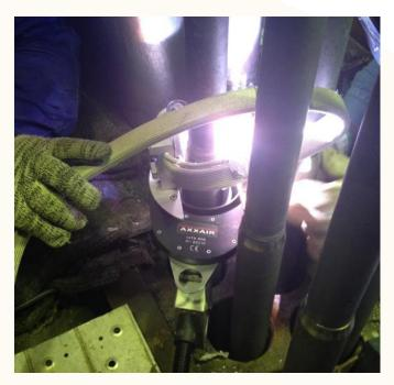
This type of machine can be used to weld carbon steel tubes.
