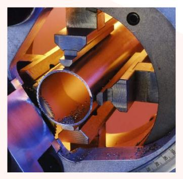
This precision is required for the welding machine to be able to close the seam and to make an adequate welding sealing.
