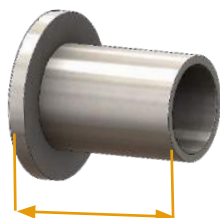
Minimal straight length of the tube: 0.5» (12.70 mm)
