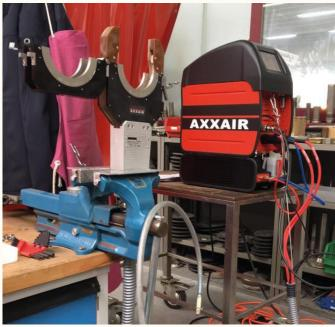
The electronics in charge of piloting the rotors of the welding heads is specifically designed to support various motor type, CD, brushless, stepping motors but also encoders or tachometers, making these power supply one of the most versatile on the market today.
