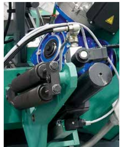
Hydraulic cylinder for bow movement
