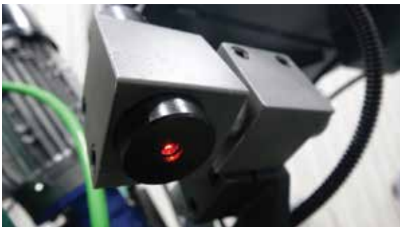
Laser pointer for cutting position
