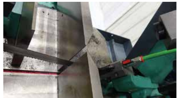
Laser pointer for cutting position
