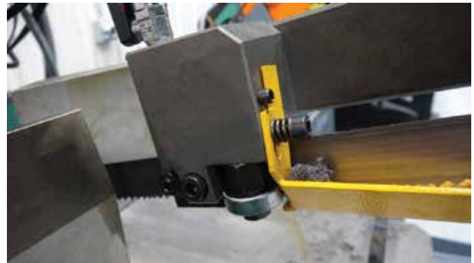
Adjustable carbide blade guides
